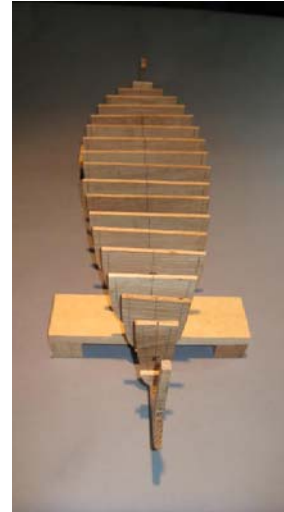
Construction jig holding keel and uncut frames
