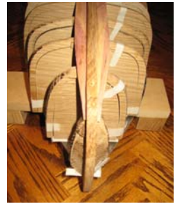
Stern view of garboards
