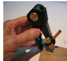
Mark the .234 inch width to cut frames
