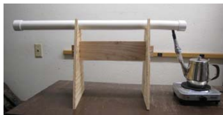
Trestle stand holding steam tube
