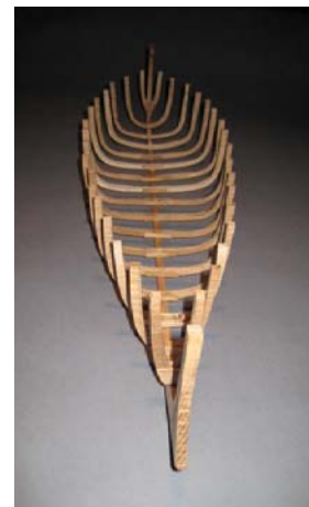
Cut frames doweled in place to keel
