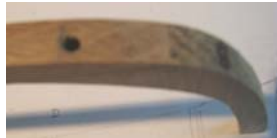
Drill #26 hole in keel scarf
